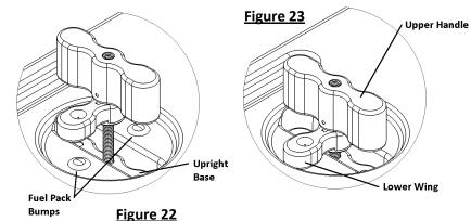
aligned with the bumps on the Fuel Pack (see **Figure 22**) until the Extension Handle is sufficiently tight and the Upper Handle and Lower Wing are perpendicular to each other (see **Figure 23**).
